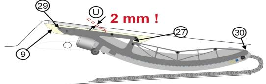
Graphic 1.10.2 Adjustment of the installation position of the ORBIS.
