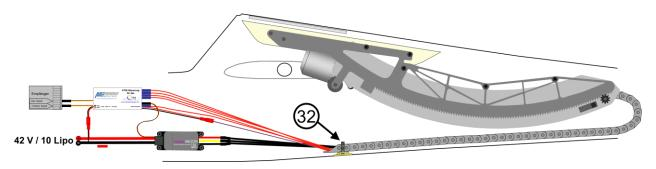
Graphic 1.11.1. Fastening of the energy chain in fuselages
