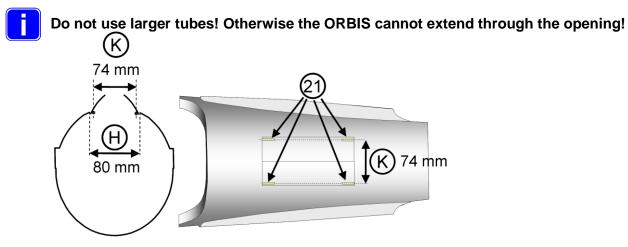
Graphic 1.7.1 Attachment of Fuselage hatch hinges
