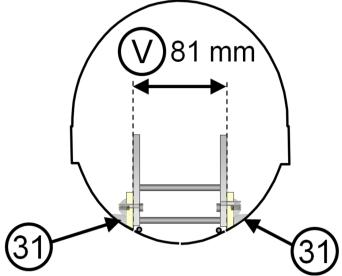
Graphic 1.10.3. Cross section of the fuselage upside down with the inserted aluminium support frame
