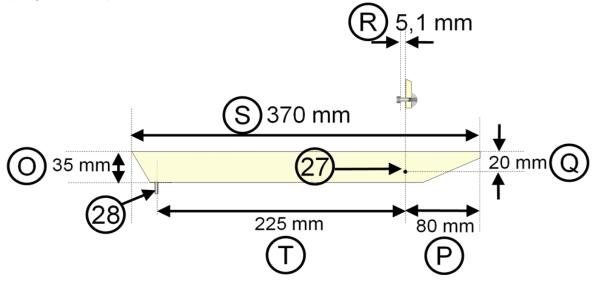
Graphic 1.10.1. Cutting out the left birch plywood support for the aluminium-support-frame
