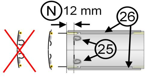
Graphic 1.9.1. Attachment of the hooks for the flap springs
