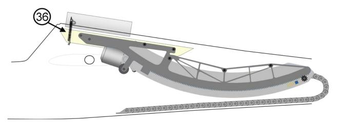
Graphic 1.17.1. Installation of springs on the fuselage hatches and a piece of wood on the left fuselage hatch
