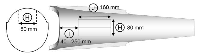
Graphic 1.6.1 Cut out the fuselage hatches
