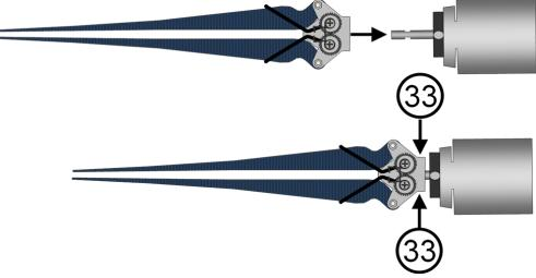
Graphic 1.15.1. Mounting of the prop mechanism
