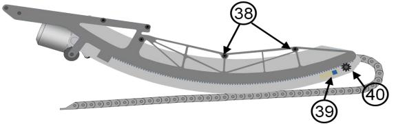
Graphic 4.2.-1. Gearwheel and limit stop for the rollerlevel switch
