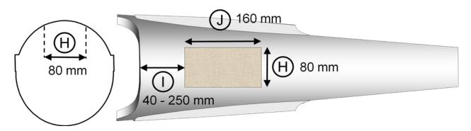
Graphic 1.5.1 Cast for a fuselage cover
