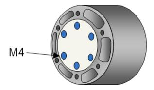
Graphic 4.1.-3. The motor bell of the Streckermotor with the M3/M4 holes
