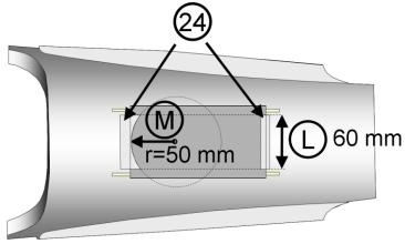
Graphic 1.8.1. Attachment of limit stop for the fuselage hatches
