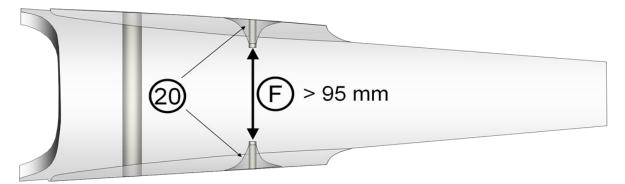
Graphic 1.4.1 Cut-back of the rear wing spar
